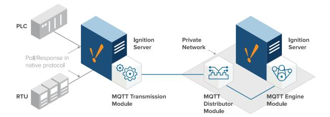
As their name suggests, edge gateways live at the outermost edge of a SCADA system. With an abundance of legacy PLCs and devices still using poll-response communication protocols, edge gateways act as a bridge to connect to these legacy devices, converting them to MQTT, enabling them to communicate to MQTT servers, and allowing enterprise networks to access the data.
