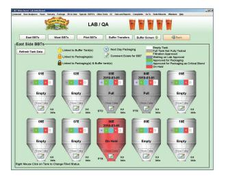
Sierra Nevada Brewery Co. built a tank status screen through FactoryPMI, which allowed the plant to coordinate its filtration to packaging workflow.
