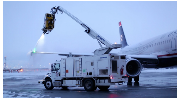
One of Global Ground Support's deicing trucks preparing an aircraft before takeoff.
